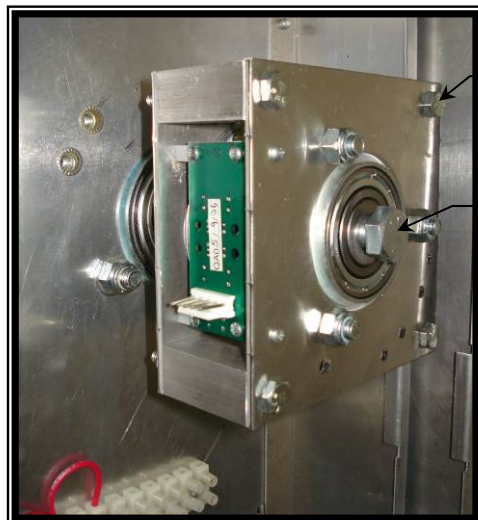
Figure 7 - Place New Encoder on Shaft
